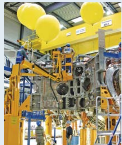
Wendelstein 7-X module 5 during installation of the bus bar system.
